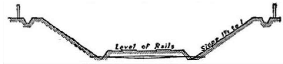
Typical Section of Railway in Cutting.
